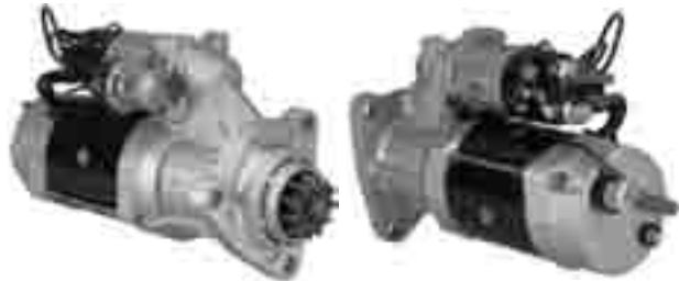
2-2366-DR Starter - Delco 39MT Series 12 Volt, CW, 11-Tooth Pinion
