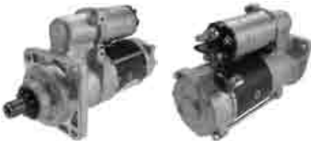
2-2389-DR (Ref# 61772N) Starter - Delco 29MT Series 12 Volt, CW, 9-Tooth Pinion
