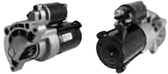
2-2638 Starter - Mitsubishi PMGR 1.7kW/12 Volt, CW, 12-Tooth Pinion
